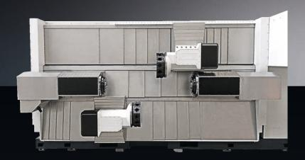
In addition, flexibly utilizable steady-rests are possible, each optionally movable in two CNC axes on a crossslide, in order to be brought quickly and precisely from a protected park position to the usage position.
