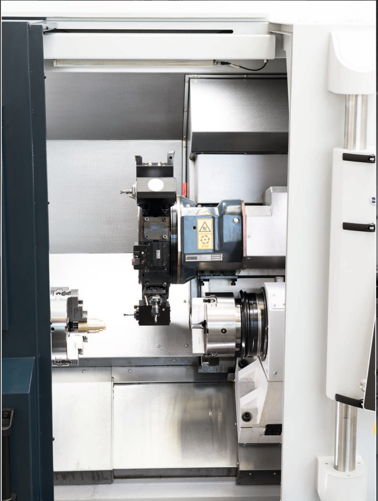
Figure shows turret disc BMT45 and subspindle
